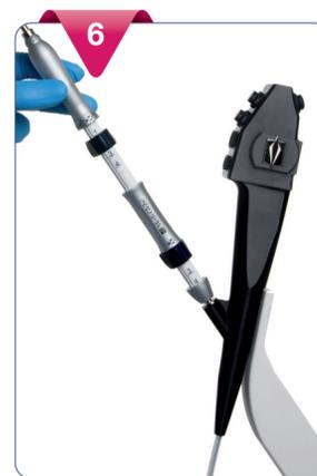
Insert the needle into the target tissue. The maximum needle projection can be preset with the upper Twist-Lock for puncture depth adjustment. Now stab into the target structure in a controlled manner.
