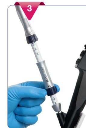
Adjust the sheath length. To do this, unlock the lower Twist-Lock (lock/unlock symbol) and slide the handle down until the desired position for the tip of the sheath is reached. Then fix the setting.
