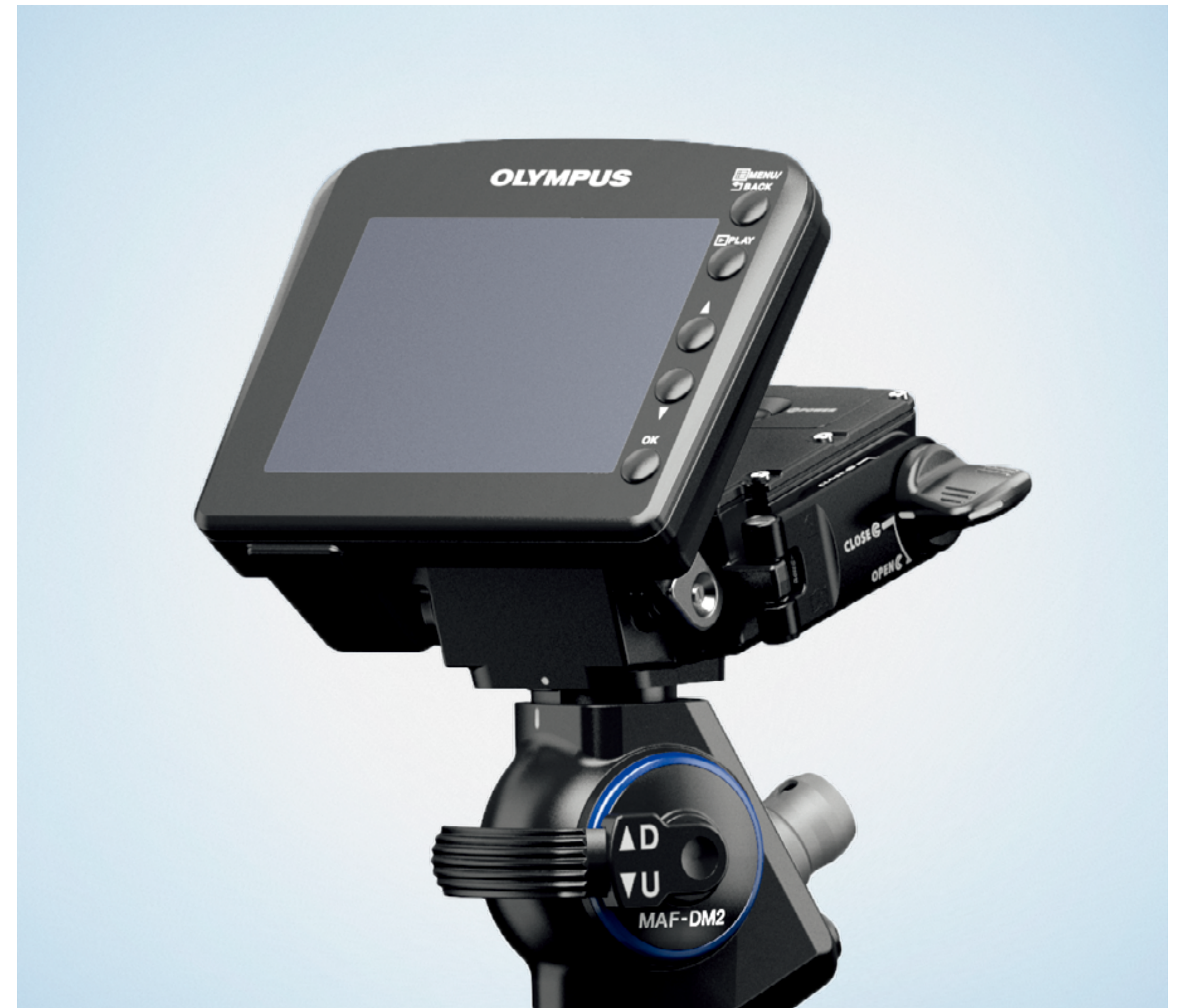
The 3.5-inch monitor can be tilted to adjust the orientation — this enables observation and control operations in a single view
